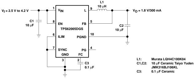
NOTE: For low noise operation connect SYNC to VIN
