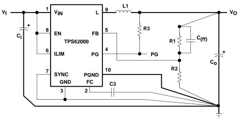
Figure 16. Layout Diagram
