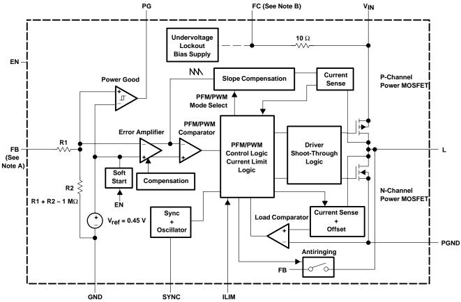
NOTES: A. The adjustable output voltage version does not use the internal feedback resistor divider. The FB pin is directly connected to the error amplifier.
