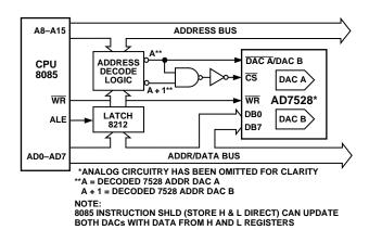
Figure 12. AD7528 Dual DAC to 8085 CPU Interface
