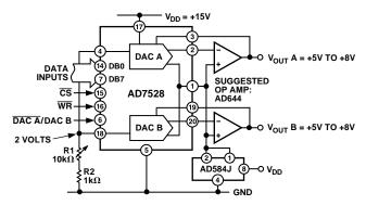
Figure 8. AD7528 Single Supply Operation
