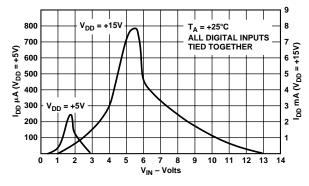
Figure 3. Typical Plots of Supply Current,  $I_{DD}$  vs. Logic Input Voltage  $V_{IN}$ , for  $V_{DD} = +5 \text{ V}$  and +15 V
