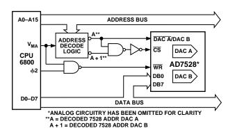
Figure 11. AD7528 Dual DAC to 6800 CPU Interface
