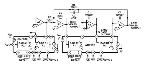
Figure 14. Digitally Controlled State Variable Filter
