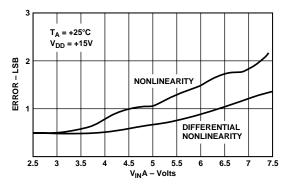
Figure 10. Typical AD7528 Performance in Single Supply Voltage Switching Mode (K/B/T, L/C/U Grades)
