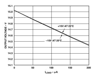
Figure 3. +15 V/-15 V Output Voltage vs. Load Current, Typical Configuration
