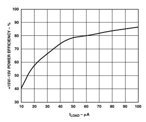
TPC 3. +15 V/-15 V Power Efficiency vs. Load Current
