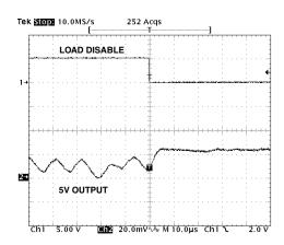
TPC 9. 5 V Output Transient Response, Load Disconnected
