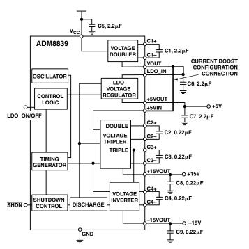
Figure 4. Current Boost Configuration
