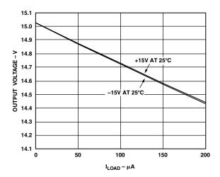
TPC 6. +15 V/–15 V Output Voltage vs. Load Current, Typical Configuration
