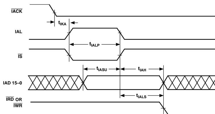
Figure 20. IDMA Address Latch
