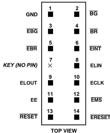
Figure 7. Target Board Connector for EZ-ICE<sup>®</sup>\*
