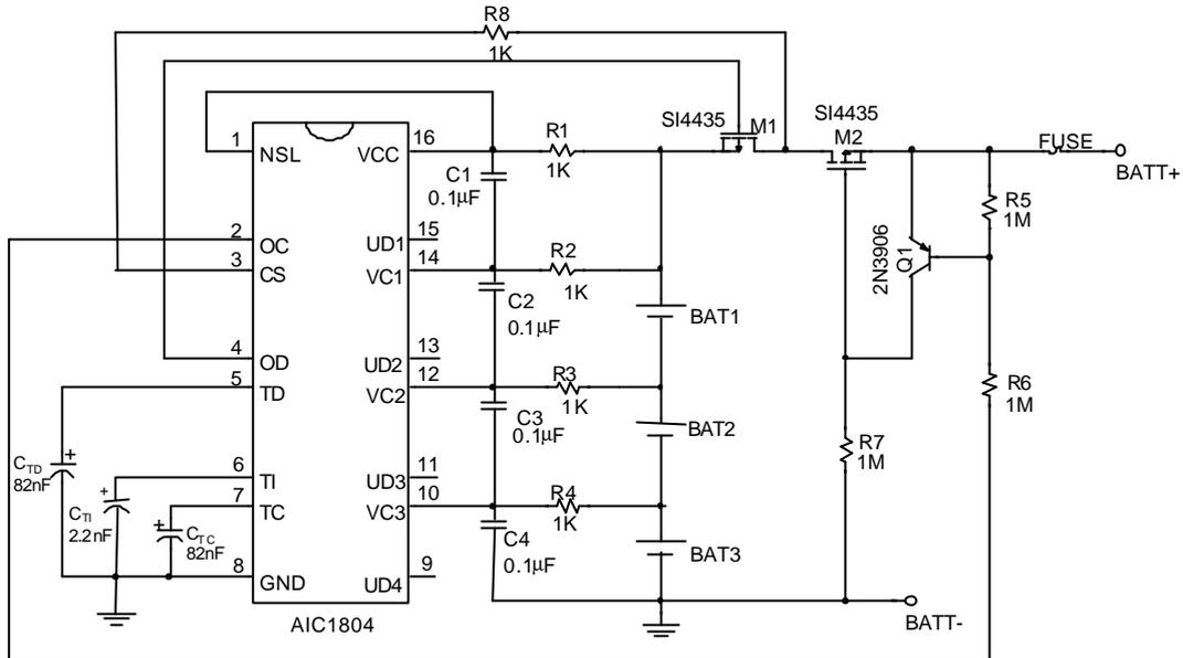
Fig. 1 Protection Circuit for Three-Cell Lithium-Ion Battery Pack
