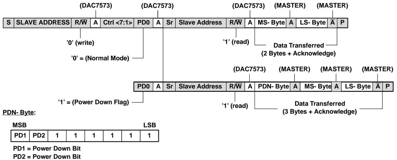
**Figure 37. Standard and Fast Mode: Slave Transmitter**
