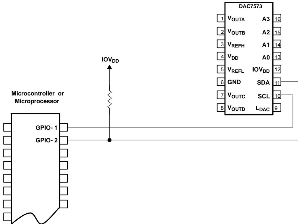
NOTE: DAC7573 power and input/output connections are omitted for clarity, except I<sup>2</sup>C Inputs.
