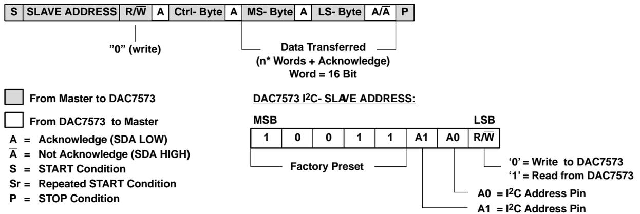
**Figure 35. Standard and Fast Mode: Slave Receiver**
