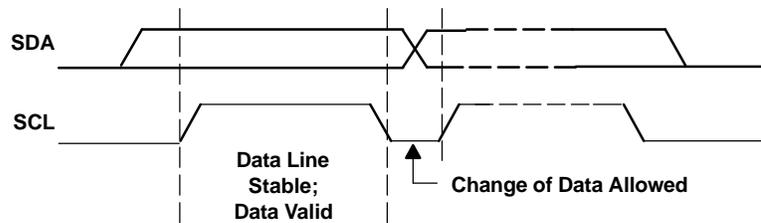
**Figure 32. Bit Transfer on the I<sup>2</sup>C Bus**
