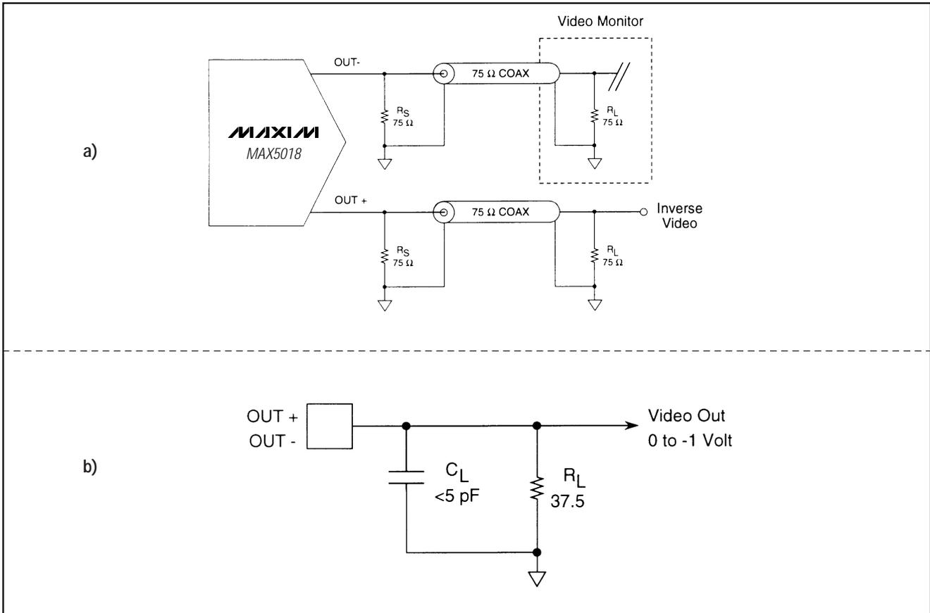
Figure 7. Standard Load (a) and Test Load (b)
