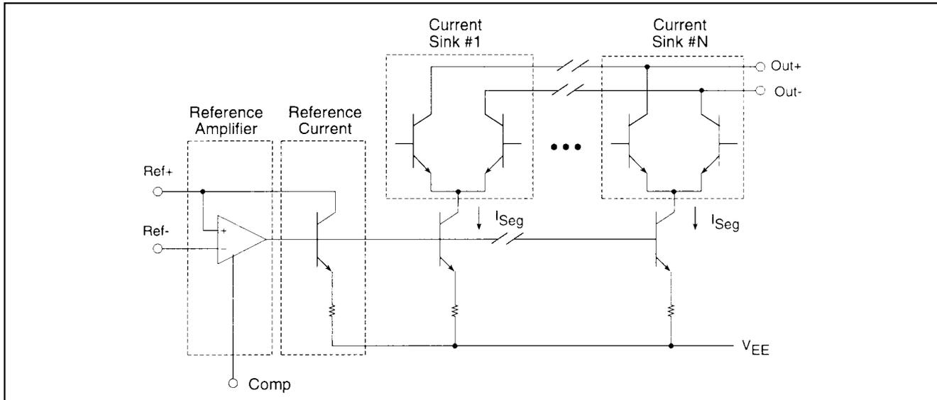
Figure 3. Reference Buffer and DAC Output Circuit
