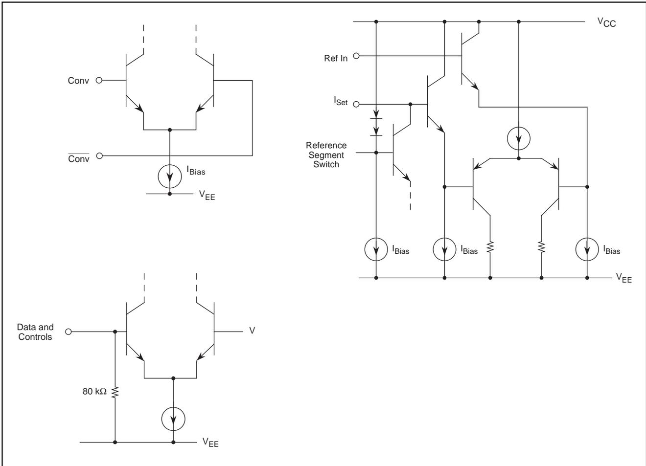
Figure 2. Equivalent Input Circuits—Data, Clock, Controls, and Reference
