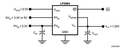
FIGURE 6. SSTL-2 Implementation with higher voltage rails
