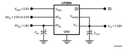
FIGURE 5. Lower Power Dissipation SSTL-2 Implementation
