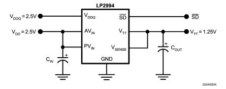
FIGURE 1. SSTL-2  $V_{TT}$  Termination
