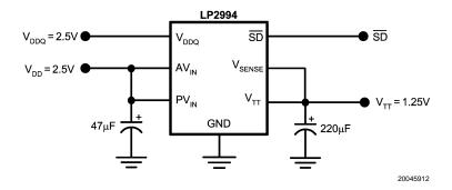
FIGURE 12. Typical SSTL-2 Application Circuit
