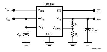
FIGURE 9. Increasing V<sub>TT</sub> by Level Shifting
