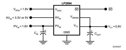
FIGURE 7. Recommended DDR-II Termination
