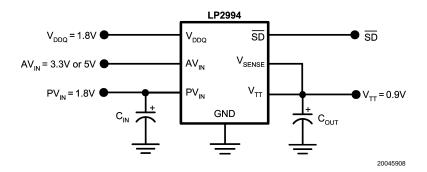
FIGURE 8. DDR-II Termination with higher voltage rails
