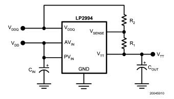
FIGURE 10. Decreasing  $V_{\rm TT}$  by Level Shifting
