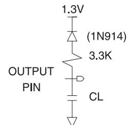
Note:  $CL = 100$  pF including jig capacitance, except for the -45 and -55 devices, where  $CL = 30$  pF.
