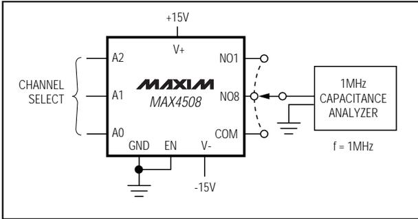
Figure 8. NO<sub>8</sub>, COM<sub>8</sub> Capacitance
