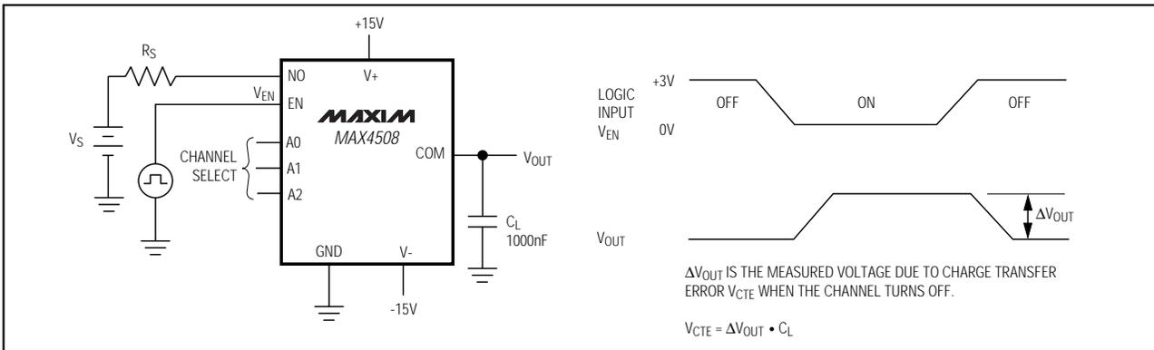
Figure 5. Charge Injection
