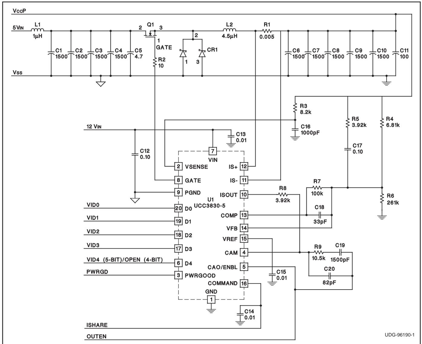
Figure 8. UCC3830 configured for 4-bit or 5-bit operation.
