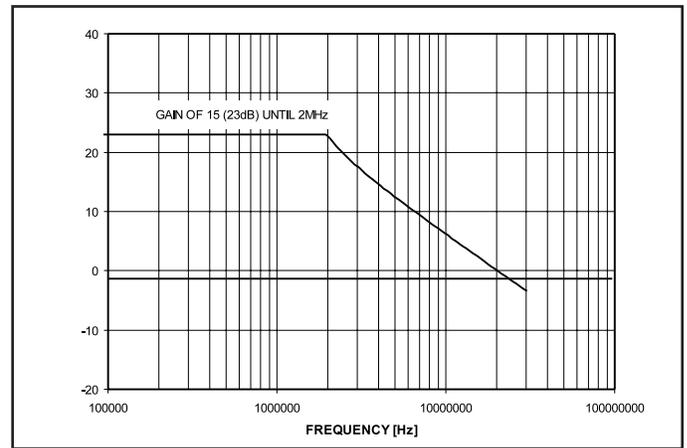
**Figure 2. Current sense amplifier gain vs frequency.**
