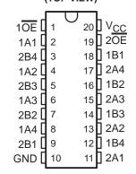
The device is organized as two 4-bit low-impedance switches with separate output-enable  $(\overline{OE})$  inputs. When  $\overline{OE}$  is low, the switch is on and data can flow from port A to port B, or vice versa. When  $\overline{OE}$  is high, the switch is open and a high-impedance state exists between the two ports.
