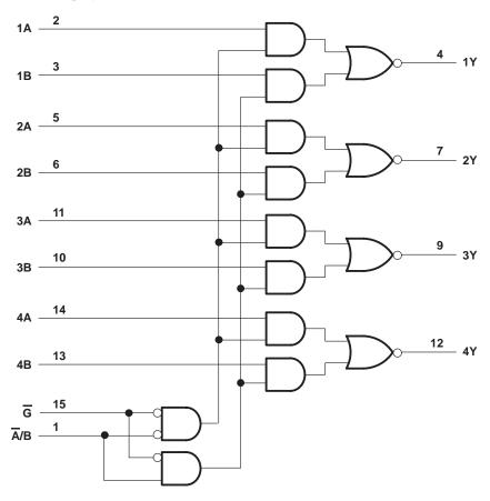
Pin numbers shown are for the D, DB, DGV, J, N, PW, and W packages.
