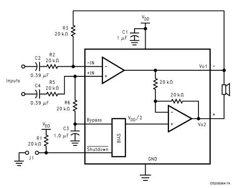
FIGURE 2. Differential Amplifier Configuration for LM4900
