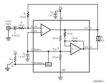
FIGURE 1. Typical Audio Amplifier Application Circuit
