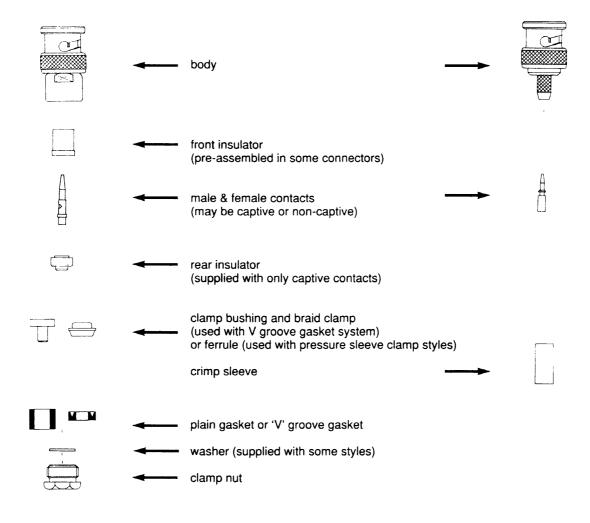
The piece parts indicated above are typical for BNC connectors. For assembly information and to assist recognition and checking of parts supplied turn to the appropriate assembly instruction page or consult our Sales Office
