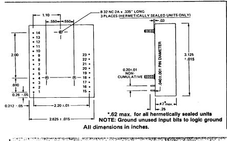
PIN ASSIGNMENTS 15 EXT. REF. 16 INT. REF. 17 · 15VDC 18 - 15VDC 19 LOGIC GROUND 20 ANALOG GROUND 21 + 15VDC 22 SIN OUT 23 COS OUT MSB (180°) BINARY INPUTS 11 12 13 LSB (.02197°) FOR INTERNAL REF. CONNECT PIN 15 TO 16 PART NUMBER DESIGNATION Add 883 for HI-REL Add H for Hermetic Seal Add D for separate logic ground Add 12 for ± 12 VDC operation Accuracy: (A = 4 minutes; B = 8.5 minutes)
