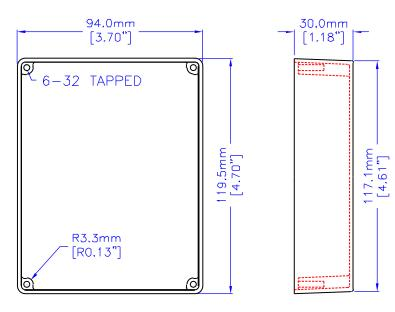
NOTE: FOR DETAIL DIMENSIONING REFER TO DRAWING # 1590BB
