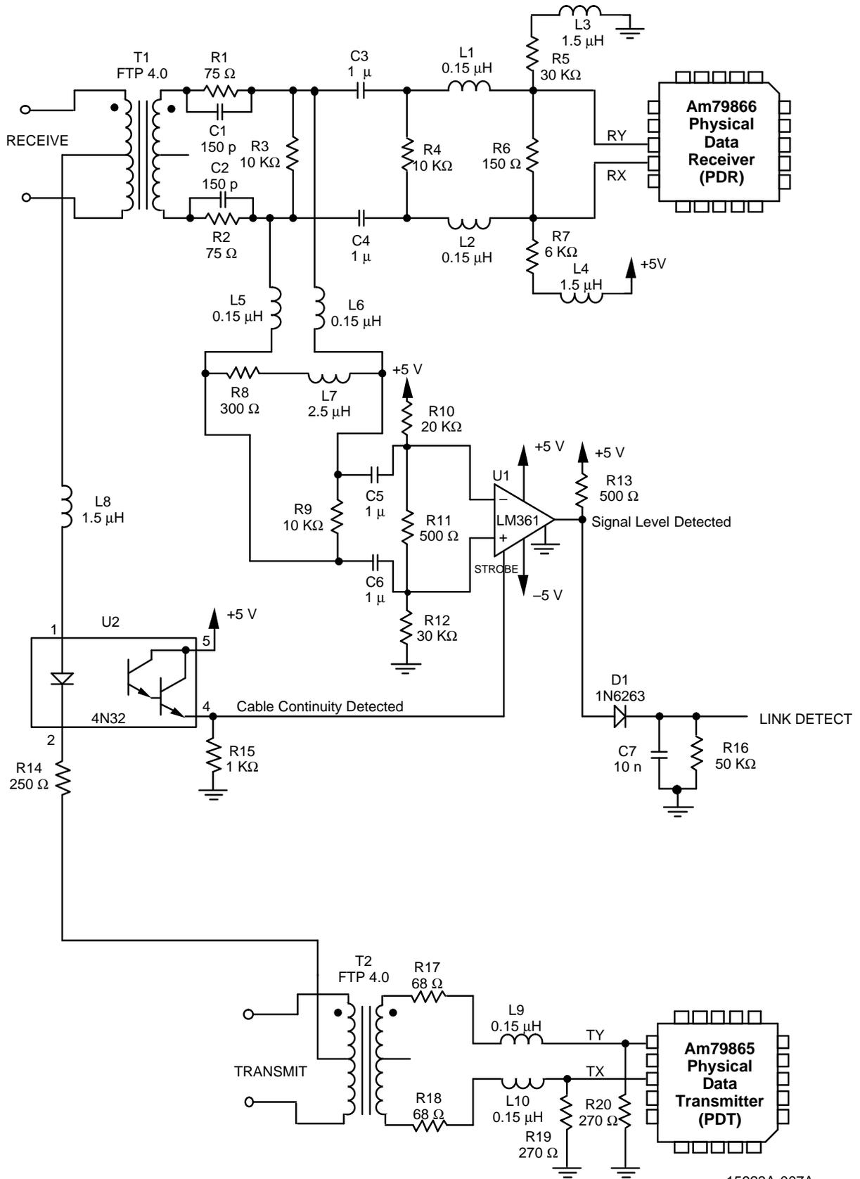
Figure 7. Alternative Schematic For the S-Port Using a Fast Comparator For Signal Detect
