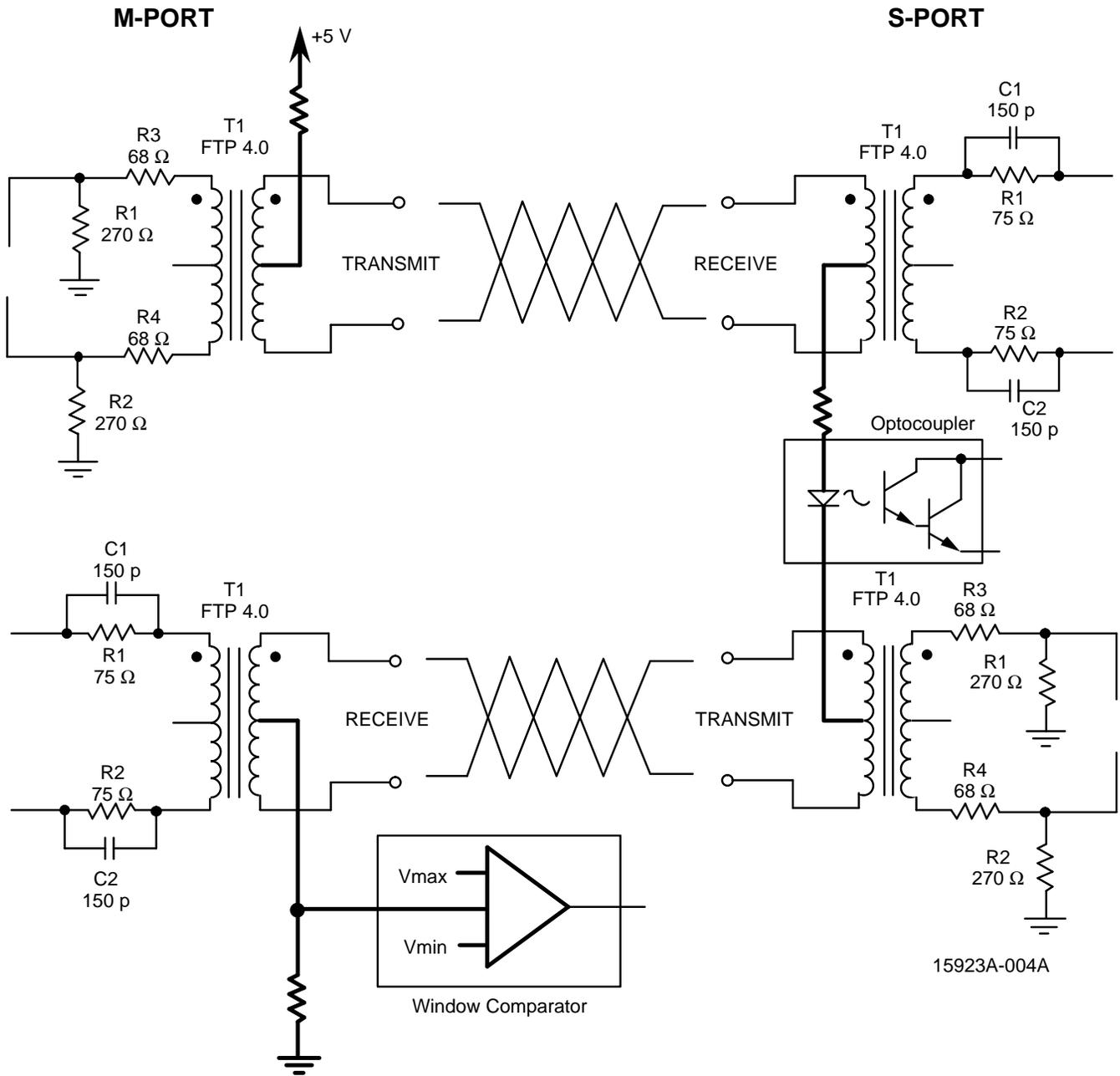
Figure 4. The Simple Option for Cable Continuity Detection
