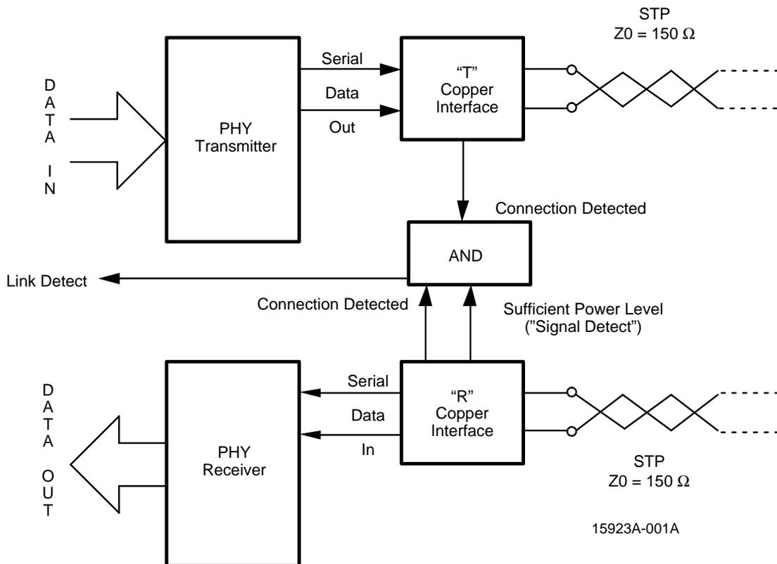
Figure 1. Block Diagram
