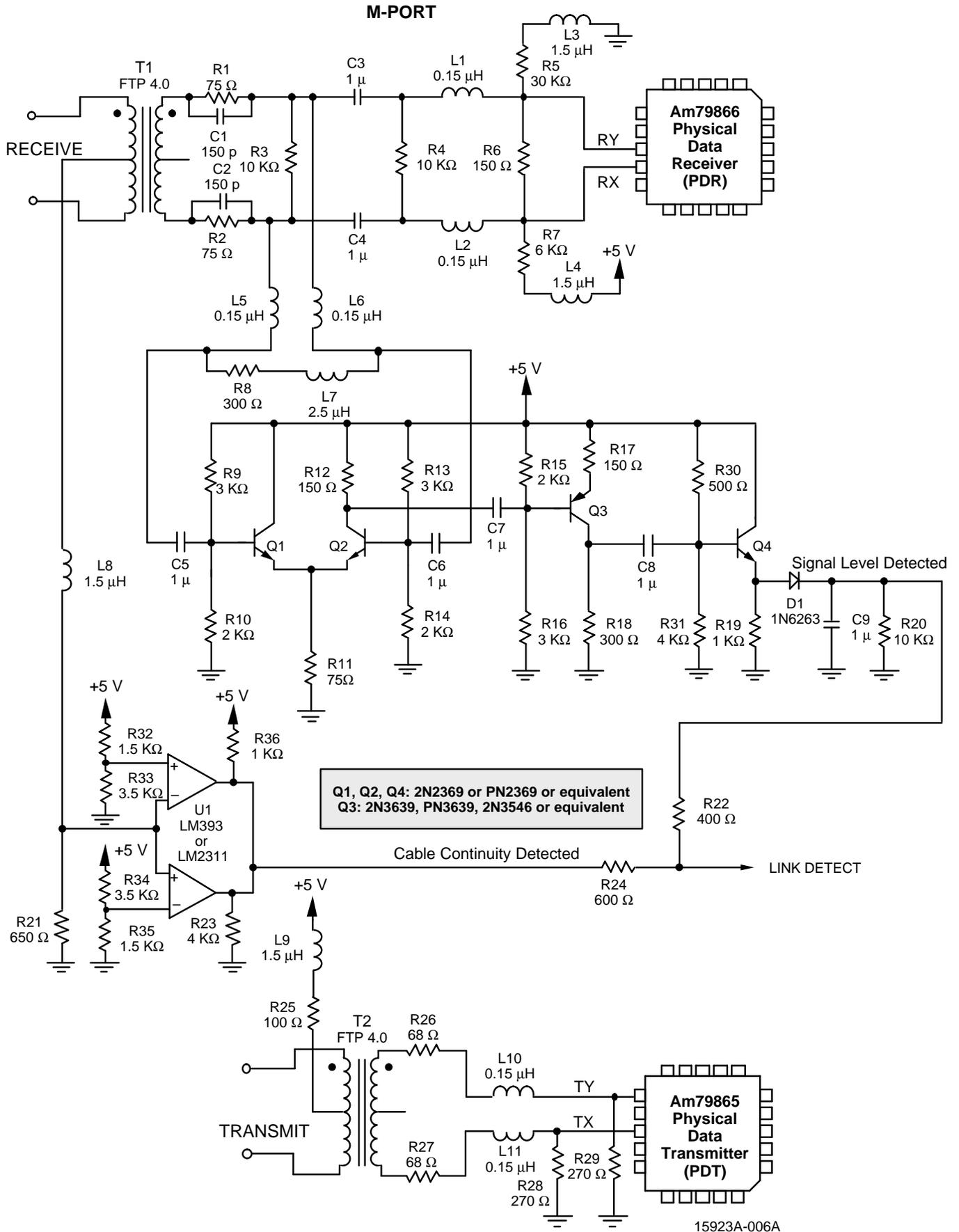
Figure 6. Schematic For the M-Port
