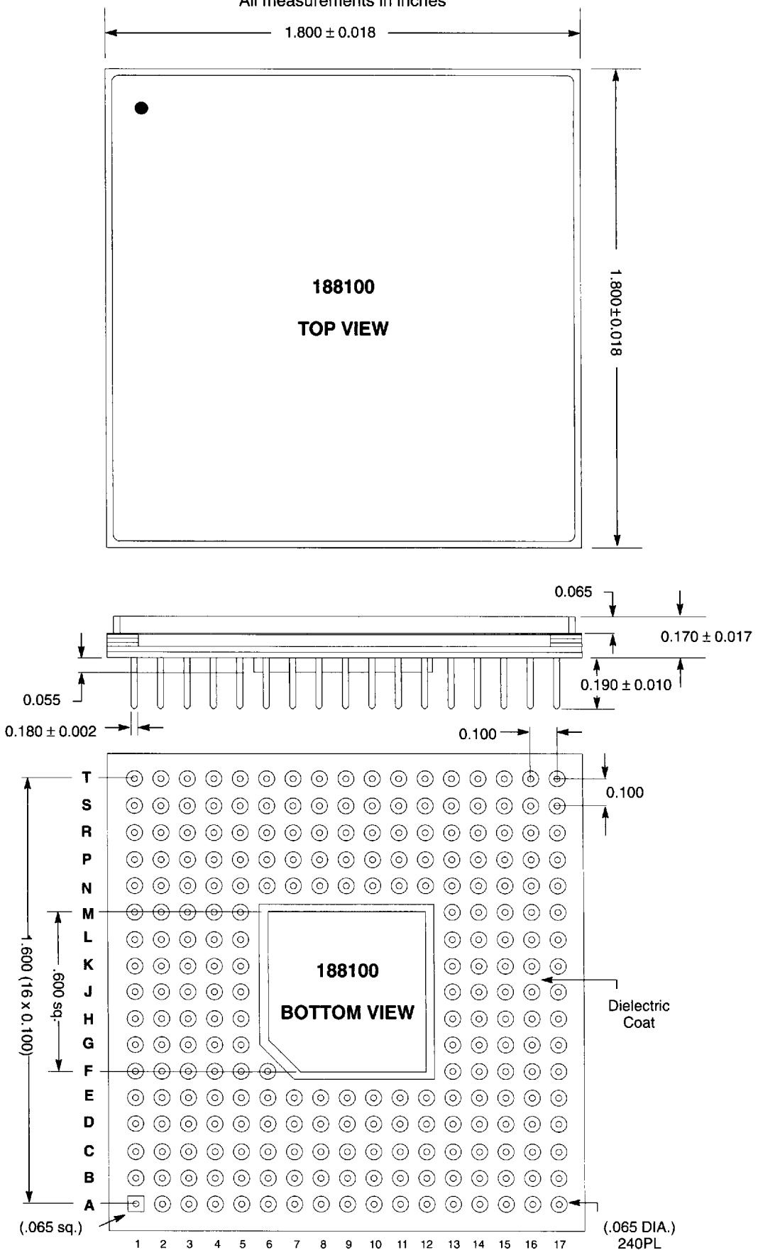
**Pin Grid Array Package**
