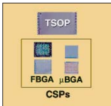
Figure 1 shows the smaller size of CSPs next to a comparable density TSOP.
