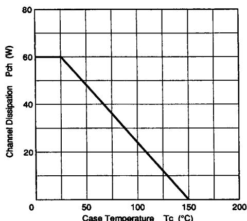
Figure 1 Power vs. Temperature Derating
