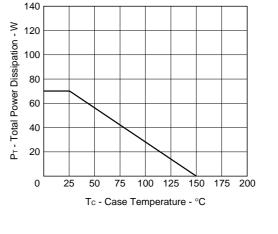
TOTAL POWER DISSIPATION vs. CASE TEMPERATURE
