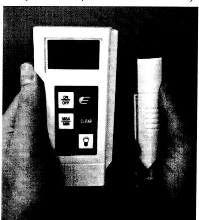
A hand held combined temperature and humidity meter. The detachable probe has a vented protection grill covering the sensors and is connected to the main unit via a 1 metre cable. Ideal for environmental monitoring or taking measurements in an air stream.
