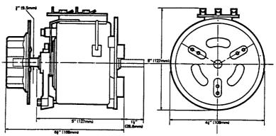
MOUNTING DETAILS—3 Holes M5 tap  $\times \frac{1}{2}$ " (13) deep on 3" (76) P.C.D. Alternative—3 Holes M5 tap  $\times \frac{1}{2}$ " (13) deep on  $2\frac{1}{12}$ " (55.5) P.C.D. DIAL FIXING—3 Holes  $\frac{1}{12}$ " (4) Dia. 120° apert on  $1\frac{1}{4}$ " (32) P.C.D.
