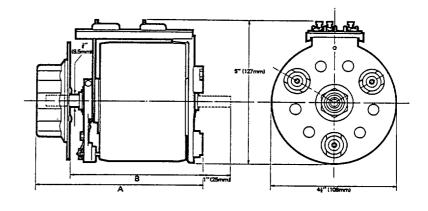
MOUNTING DETAILS -3 Holes M5 tap  $\times \frac{7}{16}$ " (11) deep on 3" (76) P.C.D. DIAL FIXING -3 Holes  $\frac{5}{2}$ " (4) Dia. 120° apart on  $1\frac{1}{2}$ " (32) P.C.D.
