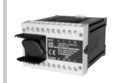
The 42000 Series DIN rail mounting power supplies are supplied ready for connection. The unit has only to be snapped on to the 35mm profile rail (DIN 46277-3) and connected to the clearly marked terminal screws. A status LED indicates power OK.
