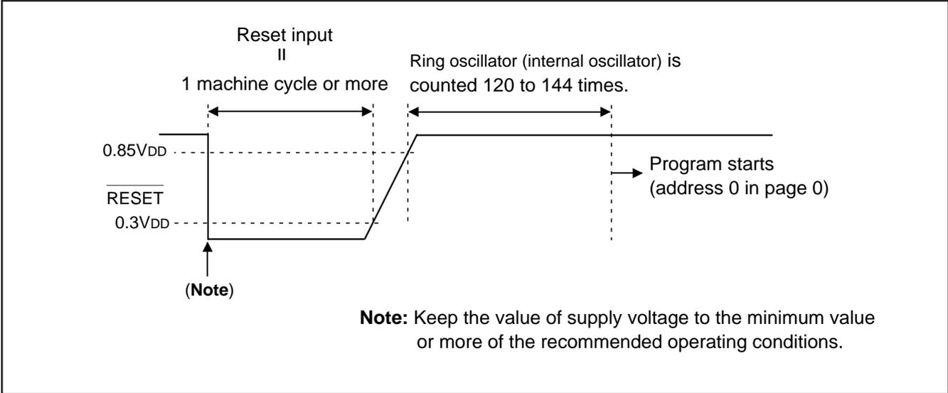
Fig. 41  $\overline{\text{RESET}}$  pin input waveform and reset operation
