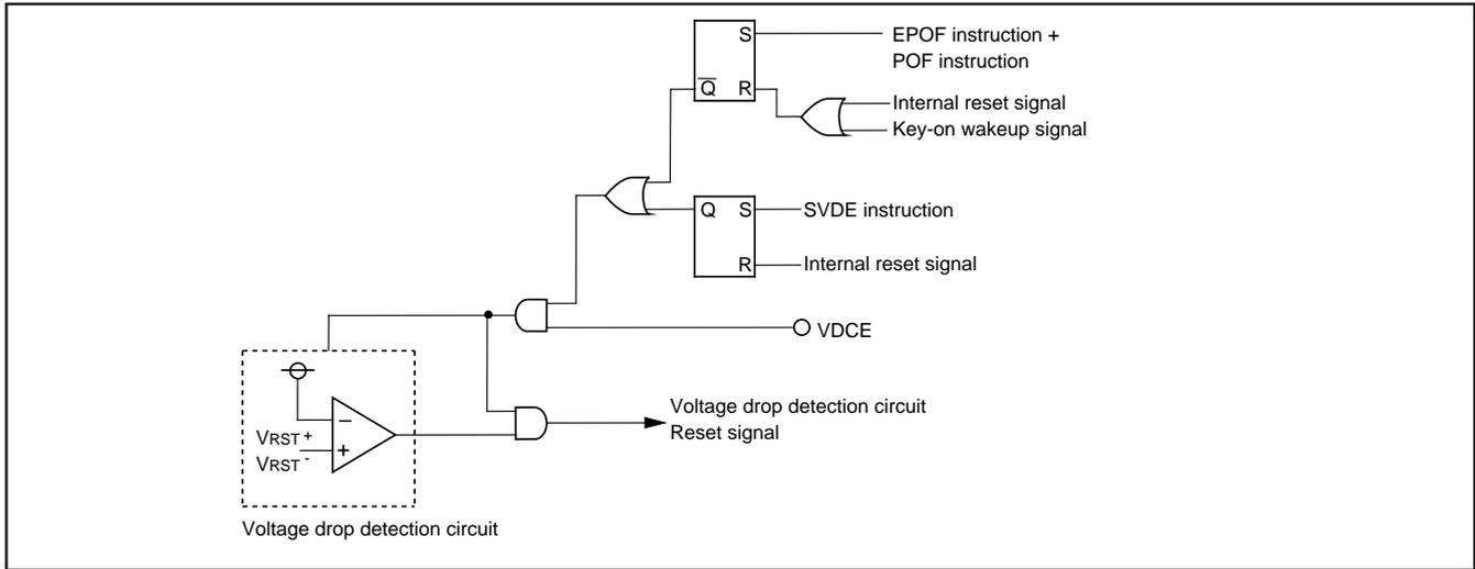
Fig. 45 Voltage drop detection reset circuit
