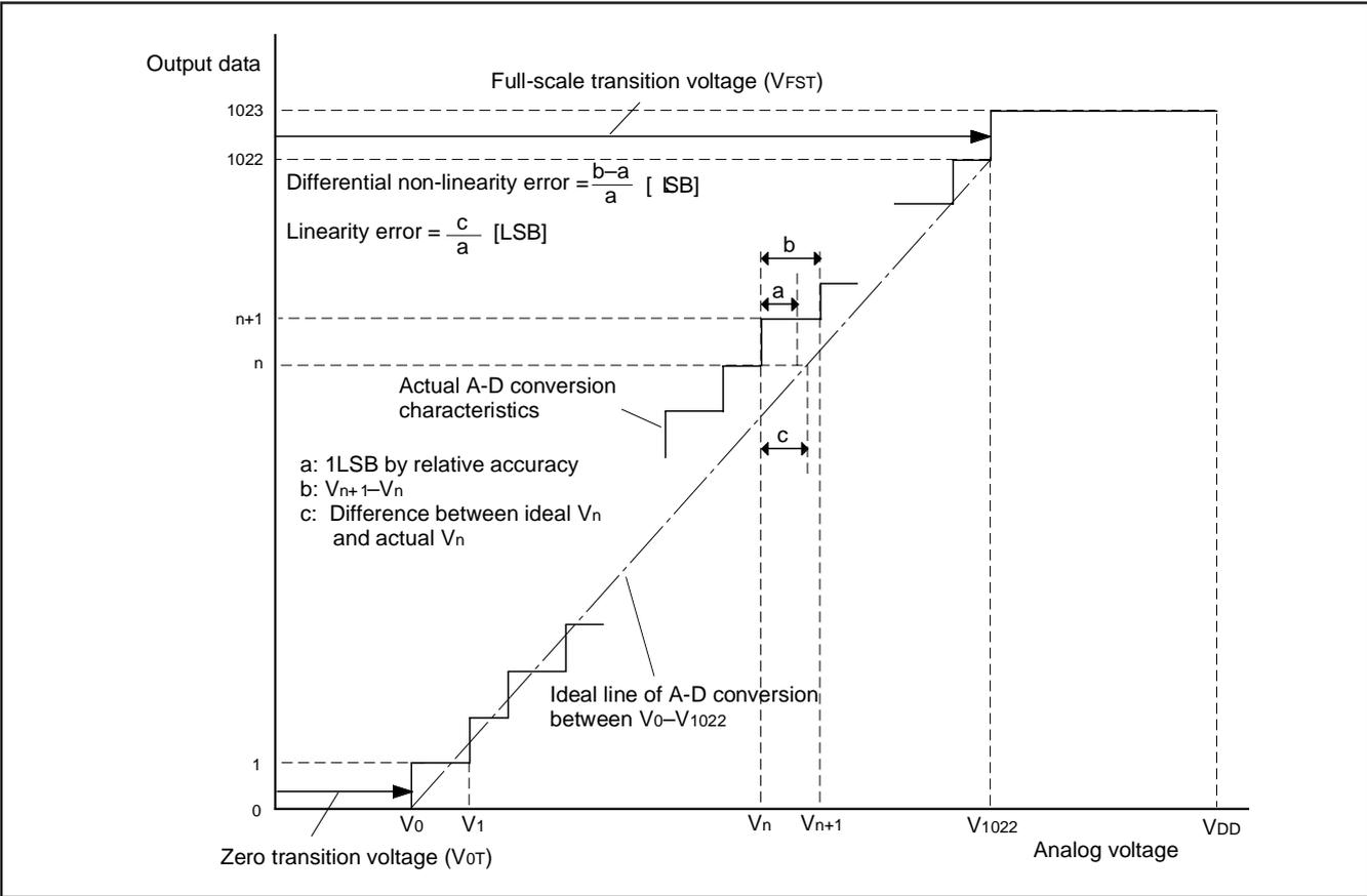
Fig. 39 Definition of A-D conversion accuracy
