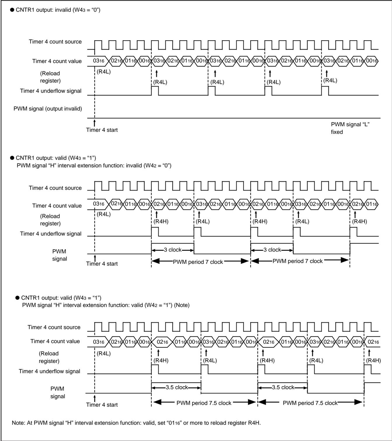
Fig. 29 Timer 4 operation (reload register R4L: "031<sub>6</sub>", R4H: "021<sub>6</sub>")
