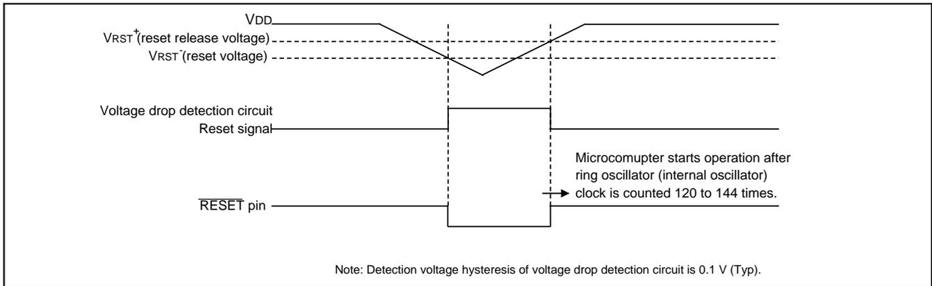
Fig. 46 Voltage drop detection circuit operation waveform
