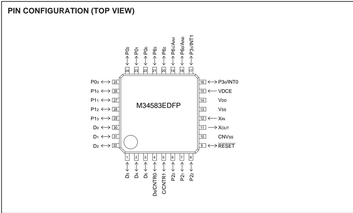
**Fig. 69 Pin configuration of built-in PROM version**
