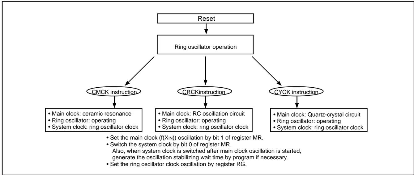
Fig. 52 Switch to ceramic resonance/RC oscillation/quartz-crystal oscillation
