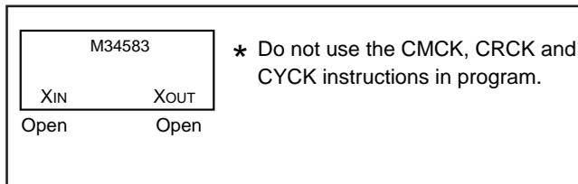
Fig. 53 Handling of  $XIN$  and  $XOUT$  when operating ring oscillator
