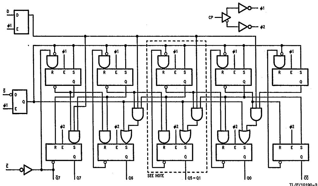
Note: Cell logic is repeated for register stages Q5 to Q1.
