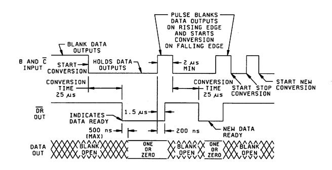
FIGURE 2. Timing waveforms.
