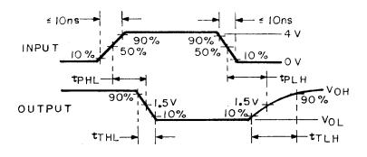
FIGURE 4. Voltage waveforms.
