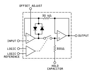
FIGURE 2. Logic diagram.
