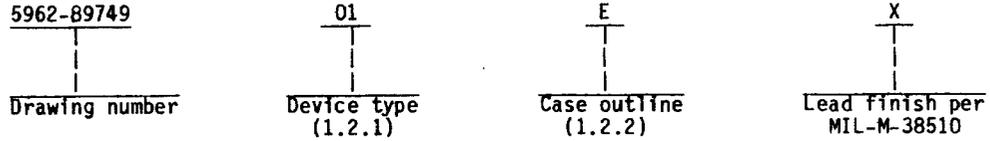
1.2.1 Device type. The device type shall identify the circuit function as follows:
