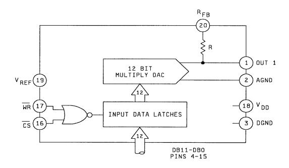
FIGURE 3. Logic diagram.
