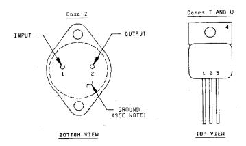
NOTE: Case is connected to ground.
