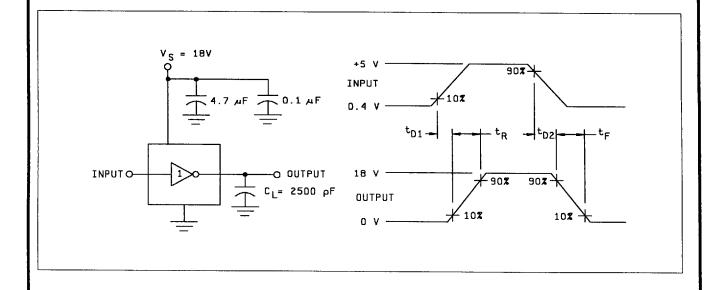
FIGURE 3. Noninverting driver switching time.
