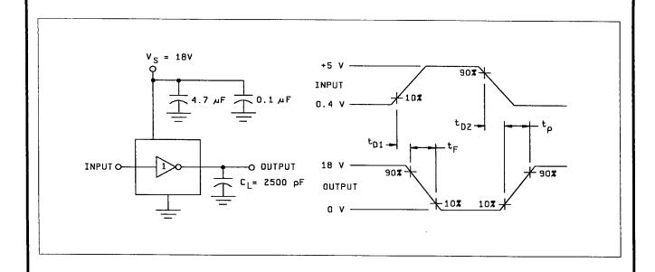
FIGURE 2. Inverting driver switching time.
