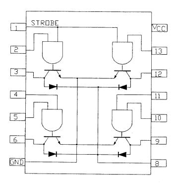
FIGURE 1. Terminal connections and logic diagram.
