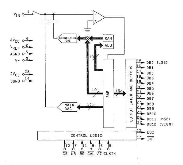
FIGURE 3. Logic diagram. (device types 01and 02)
