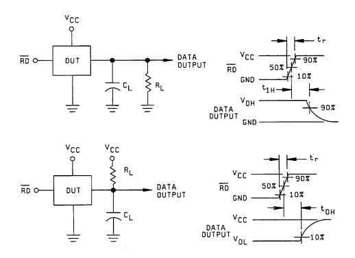
FIGURE 4. Three state test circuit and waveforms.
