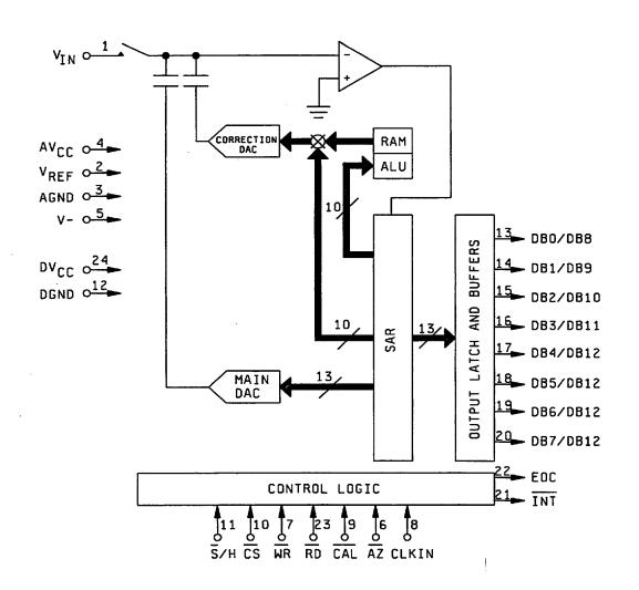
FIGURE 3. Logic diagram - continued. (device types 03nd 04)
