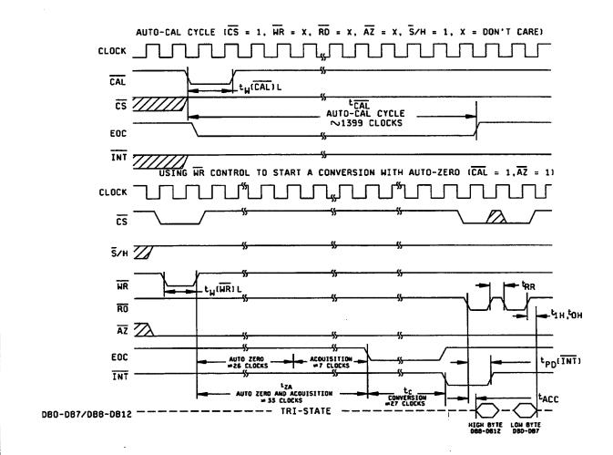
FIGURE 5. <u>Timinia diagram</u> - continued. (device types 03 and 04)
