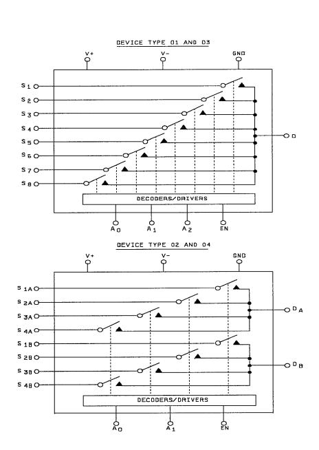
FIGURE 3. Block diagram.
