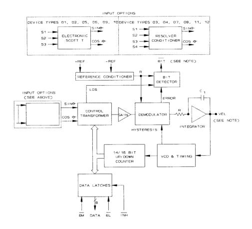
NOTE: BIT is not connected on device types 01, 03, 05, 07, 09, and 11. VEL is not connected on device types 02, 04 06, 08, 10, and 12.
