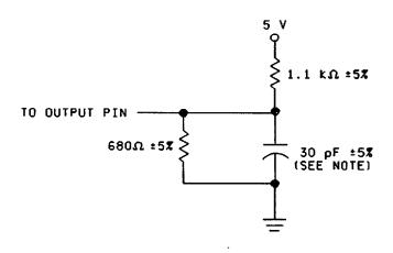
NOTE:  $C_L$  includes scope and jig capacitance.
