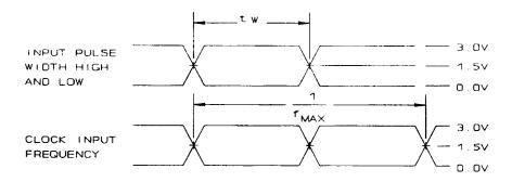
FIGURE 5. Switching waveforms and test circuits.
