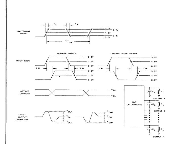
$C_L$  = 47 pF -0 percent, +20 percent chip capacitor plus  $\ge$  3 pF of equivalent capacitance from the test jig and probe.  $R_L$  = 450  $\Omega$  ±1 percent, chip resistor in series with a 50 $\Omega$  termination. For monitored outputs, the 50 $\Omega$  termination shall be the 500 characteristic impedance of the coaxial connector to the oscilloscope. Input signal to the device under test:
