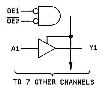
FIGURE 3. Logic diagram.
