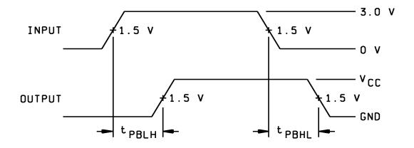
FIGURE 3. Switching test circuit and waveforms.
