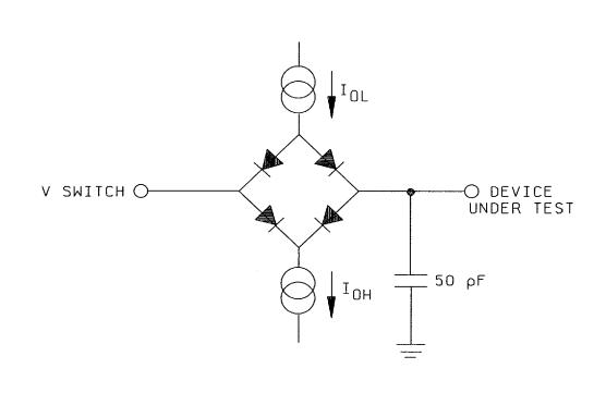
FIGURE 3. Switching test circuit and waveforms.
