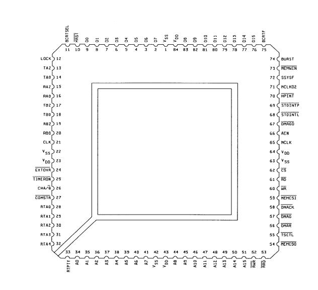
NOTE: MEMWIN is an internal test pin only and should be considered a floating pin and not for use.
