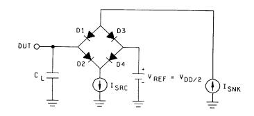
1/  $C_L$  = 50 pF minimum or equivalent (includes test jig and probe capacitance). 2/  $I_{SRC}$  is set to -1 mA and  $I_{SNK}$  is set to 1 mA for  $t_{PHL}$  and  $t_{PLH}$  measurements. 3/ Input signal from pulse generator:  $V_{IN}$  = 0.0 V to  $V_{DD}$ ;  $f \le 10$  MHz;  $t_I$  = 1.0 V/ns ±0.3 ns/V;  $t_I$  and  $t_I$  shall be measured from 0.1  $V_{DD}$  to 0.9  $V_{DD}$  and from 0.9  $V_{DD}$  to 0.1  $V_{DD}$ , respectively.
