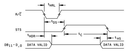
LOW PULSE FOR R/C - OUTPUTS ENABLED
