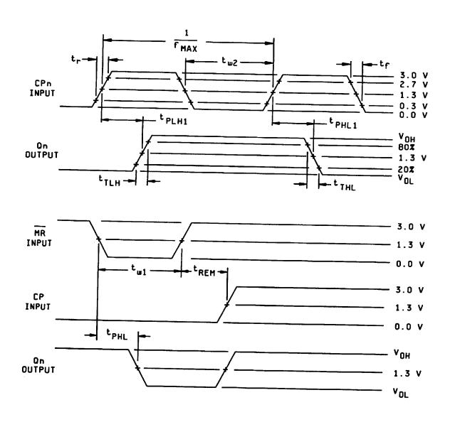
FIGURE 4. Switching waveforms and test circuit.
