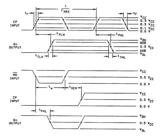
FIGURE 4. <u>Switching waveforms and test circuit</u>.
