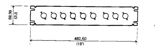
MATERIAL :- ALUMINIUM SHEET 2,0mm THICK
