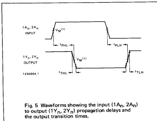
Fig. 5 Waveforms showing the input ( $1A_n, 2A_n$ ) to output ( $1Y_n, 2Y_n$ ) propagation delays and the output transition times.
