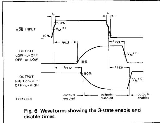
Fig. 6 Waveforms showing the 3-state enable and disable times.
