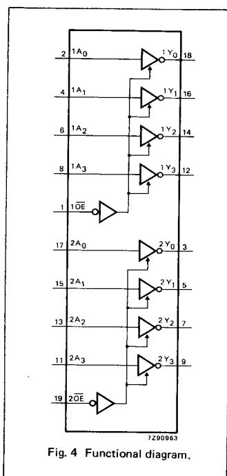
Fig. 4 Functional diagram.
